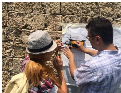
Figure 7: ESR 5 performing data acquisition with ground penetrating radar: fortification surface with alveolation decay.
